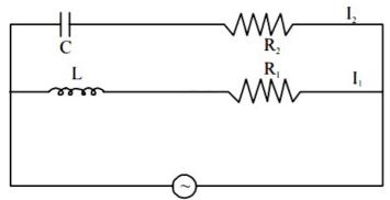
In the above circuit,  $C = \frac{\sqrt{3}}{2}\mu F$ ,  $R_2 = 20\Omega$ ,  $L = \frac{\sqrt{3}}{10}H$  and  $R_1 = 10\Omega$ . Current in L –  $R_1$  path is I<sub>1</sub> and in C –  $R_2$  path it is I<sub>2</sub>. The voltage of A. C source is given by, V =  $200\sqrt{2} \sin(100 \text{ t})$  volts. The phase difference between I<sub>1</sub> and I<sub>2</sub> is :
