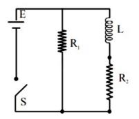
An inductor of inductance L = 400 mH and resistors of resistance  $R_1 = 2\Omega$  and  $R_2 = 2\Omega$  are connected to a battery of emf 12V as shown in the figure. The internal resistance of the battery is negligible. The switch S is closed at t = 0. The potential drop across L as a function of time is [2009]
