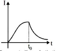
The current will grow for the time t = 0 to  $t = t_0$  and after that decay of current takes place.
