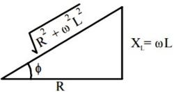
Net impedance of circuit Z =  $\sqrt{X_L^2 + R^2}$ Power factor,  $\cos \phi = \frac{R}{Z}$  $\Rightarrow \cos \phi = \frac{R}{\sqrt{R^2 + \omega^2 L^2}}$
