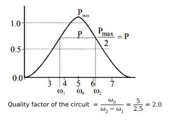
In a series L - C -R circuit,  $C = 10^{-11}$  Farad,  $L = 10^{-5}$  Henry and R = 1000hm, when a constant D.C. voltage E is applied to the circuit, the capacitor acquires a charge  $10^{-9}$ C. The D. C. source is replaced by a sinusoidal voltage source in which the peak voltage E<sub>0</sub> is equal to the constant D.C. voltage E. At resonance the peak value of the charge acquired by the capacitor will be : [Online April 22, 2013]
