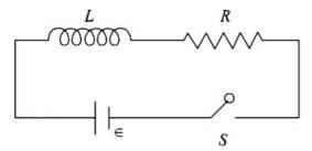
As shown in the figure, a battery of emf  $\in$  is connected to an inductor L and resistance R in series. The switch is closed at t = 0. The total charge that flows from the battery, between t = 0 and t = t<sub>c</sub>(t is the time
