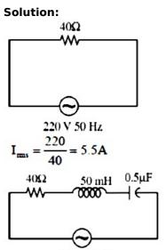
220 V 50 Hz  $\rm X_L$  is not equal to  $\rm X_C.$  So rms current in (b) can never be larger than (a).
